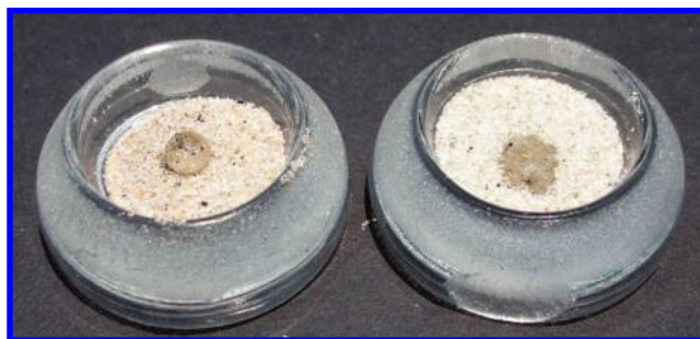
Figure 1. Water droplets placed on hydrophobic (left) and nonhydrophobic (right) sands. Note rounded drop on hydrophobic sand compared to completely absorbed water on nonhydrophobic sand [video showing water droplet on nonhydrophobic sand followed by hydrophobic sand located at http://www.northinlet.sc.edu/resource/vitex_files/aug05/Hydro1.wmv (Charles A. Gresham)].
